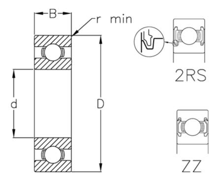
$\begin{array}{lll} B & = 6 \\ d & = 12 \\ D & = 24 \\ Dynamic load C (kN) & = 2.89 \\ Max rpm greased & = 27000 \\ Max rpm oil lubricated = 32000 \\ r min & = 0.3 \\ Static load C0 (kN) & = 1.46 \\ \end{array}$
